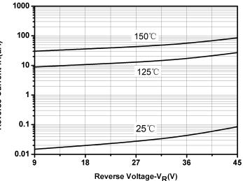
**Fig.2-Typical Reverse Characteristics**
