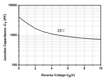
Fig.3-Capacitance vs. Reverse Voltage
